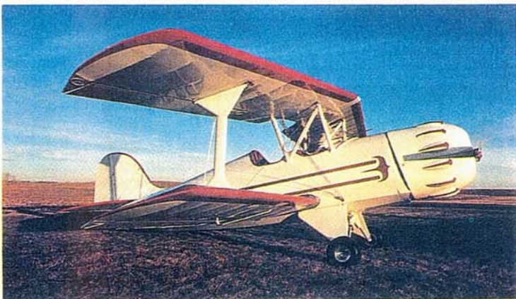
Ray Nichol's Murphy Renegade — no ribstitching or surface taping
